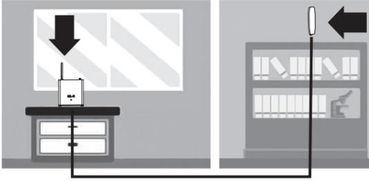
Attach the Whip and Patch antennas accordingly.
