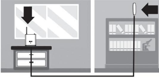
Attach the Whip and Patch antennas accordingly.
