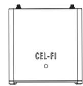
Plug-in the unit to power. The LED on the front will blink during setup.
